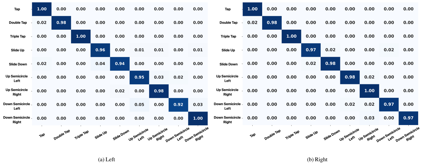
Fig. 5: Confusion matrices of the gesture classification on the left and the right surfaces.
